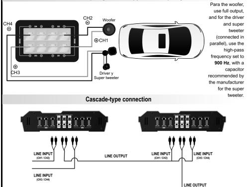
A cascade-type connection is made by transferring the first amplifier signal through the LINE OUTPUT to a second amplifier, using a duplicator, by connecting it to its ILINE INPUTS. The quantity of amplifiers that can be connected this way depends on the distance between them, the quality of the audio signal and the quality of the signal cable being used.
