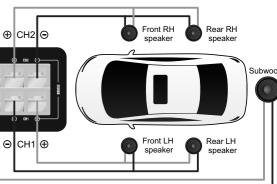
For the front and rear loudspeakers, use the high-pass frequency set to 80 Hz (at least) and for the subwoofer. use the low-pass frequency set to 80 Hz (at least).
