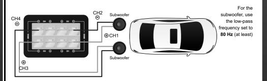
4 // Control Trio - Woofer (Bridge CH1/CH2) y Driver/ST (Bridge CH3/CH4)
